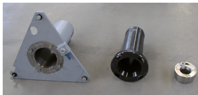
Fig 15: Nozzle holder, inner sleeve and nozzle
