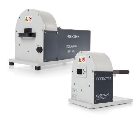
During the production process of steel, hard metals and powder metallurgical components magnetic values such as coercive field strength HcJ, weight-specific saturation polarization os and the volume-specific saturation polarization Js correlate to a variety of important process parameters and material properties.
