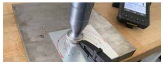
Fig. 1: Hardness measurement on sheet metal
